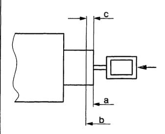
Checking solenoid switch
